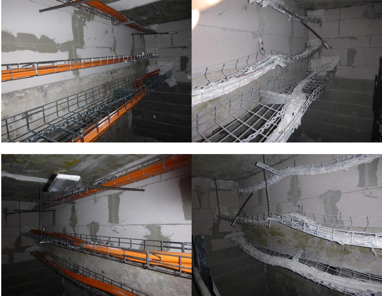
As the photos show, the structure of the EASYCONNECT trays that were tested, as well as the supports, did not collapse and they did not fully or partially come apart in any instance.
